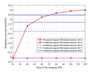
Fig. 5. WSR versus the size of the irregular RIS.  $P_{\rm T} = 10$  dBm, N = 20, K = 4.
