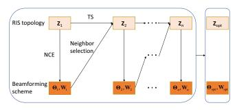
Fig. 2. The proposed joint optimization framework.
