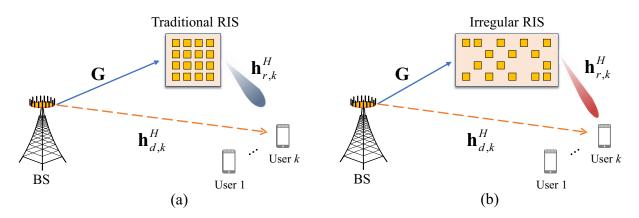
Fig. 1. The RIS-aided communication system: (a) Traditional regular RIS; (b) Proposed irregular RIS.
